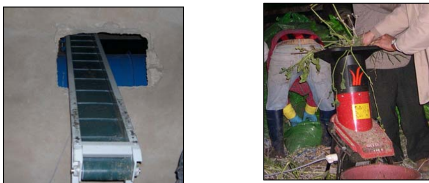
Figure 1: Shredding device in operation and the employed conveyor belt for loading the input material to the bioreactor
