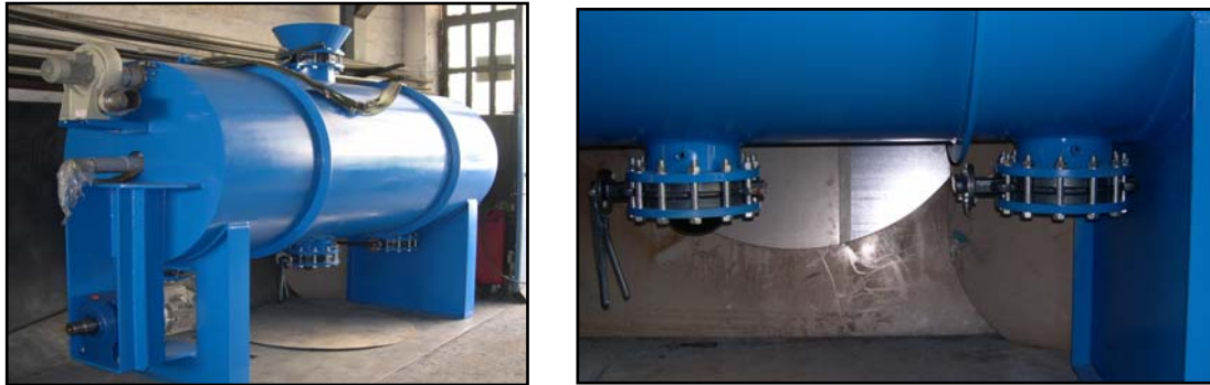
Figure 2: Compost collection portals & leachate removal system
