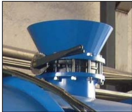
Figure 2: Supply portal for loading the input material into the bioreactor
