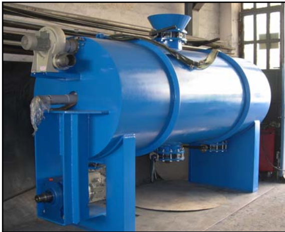
Figure 2: Supply portal for loading the input material into the bioreactor
